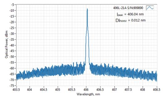
Typical spectrum of 406 nm diode laser. Measured with 10 pm resolution.
