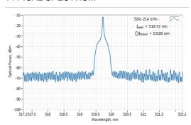
Typical spectrum of 0520 nm diode laser. Measured with 20 pm resolution.
