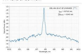
Typical spectrum of 0638 nm diode laser. Measured with 20 pm resolution.
