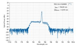
Typical spectrum of 0785S-41A nm diode laser. Measured with 10  $\mbox{pm}$  resolution.
