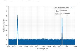
Typical spectrum of 1319 nm DPSS laser. Measured with 20 pm resolution.
