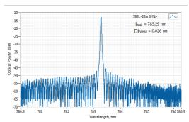
Typical spectrum of 0783 nm diode laser. Measured with 20 pm resolution.
