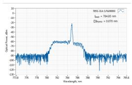
Typical spectrum of 0785S-41A nm diode laser. Measured with 10 pm resolution.
